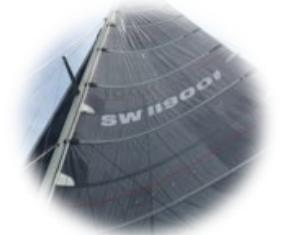
**Big Rig:** Tall double spreader rig allows for a higher aspect mainsail and jib.
