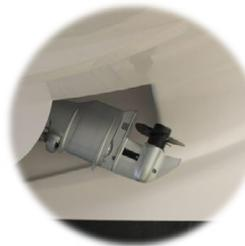
**Outboard Engines:** Reduced weight and drag, twin 20hp Honda Outboards are standard on the Sport which also has the added benefit of reduced maintenance and associated costs.
