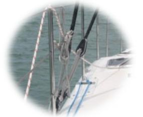
**Synthetic Rigging & Safety Lines:** Using racing technology with Dynux synthetic rigging, weight has been taken out of the rig up high.
