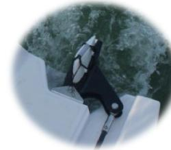
**Daggerboards and Rudders:** Improved pointing to windward (5-7 degrees), reduced drag and light, responsive steering.
