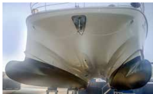
Right: Bow pods provide performance – and are a bolt-on replacement if damaged.
