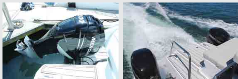
Plenty of torque and speed from these 300hp 6 cylinder Mercury outboards. Image Kevin Green
