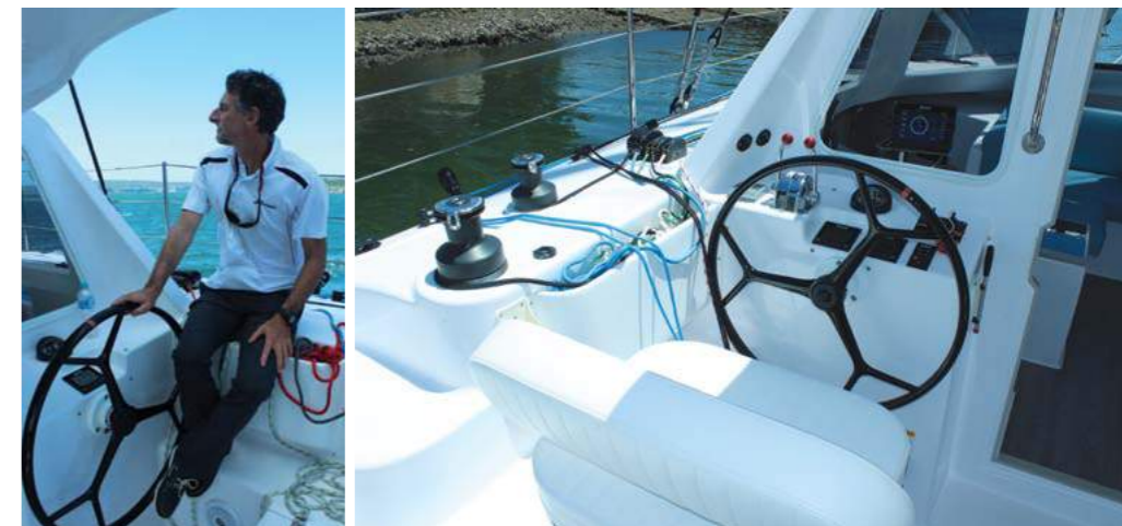
Functional twin binnacles with composite wheels work well on the 1190. Image Kevin Green
