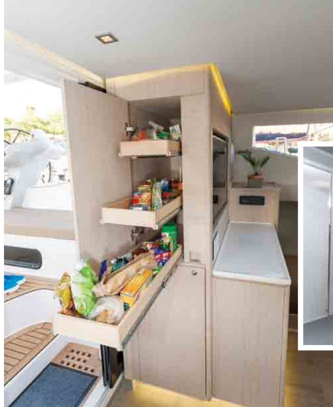
LEFT: Simple but effective joinery on the sliding cabinetry. Image Seawind
