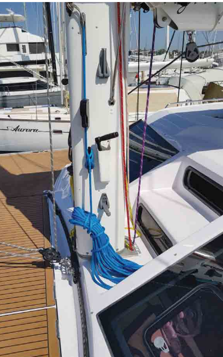
LEFT: Nearly all lines run aft and note the moulded steps for easy access to the boom. Image Kevin Green
