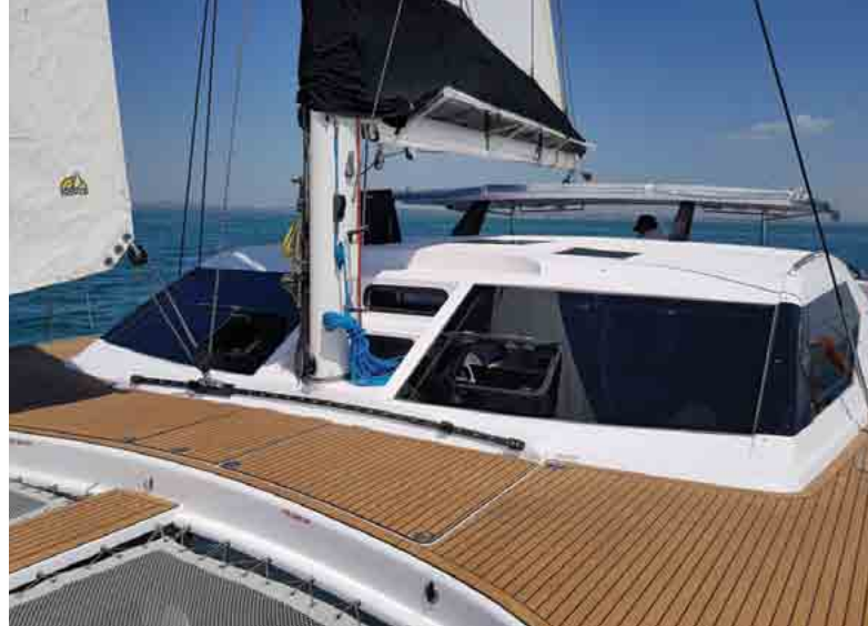
A smooth topside profile reduces windage while wide decks with Flexiteek nicely complete the Seawind 1600's topsides. Image Kevin Green
