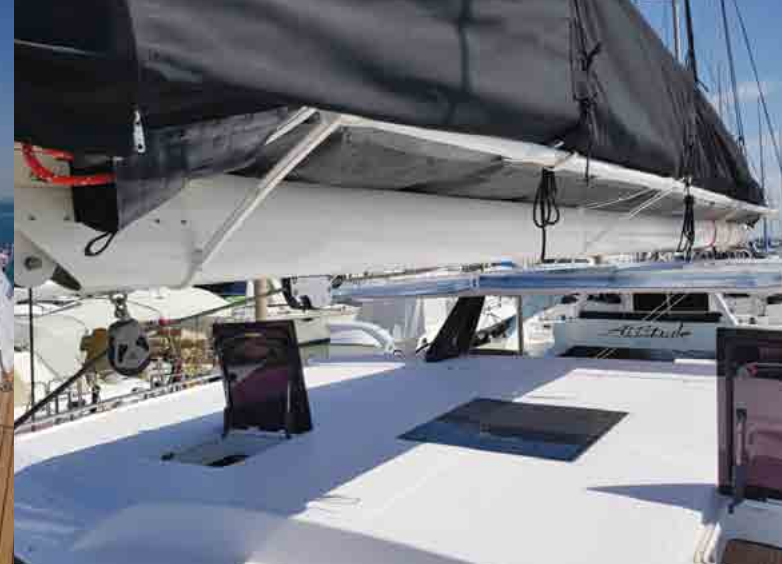
A boom gantry extension on each side is a lightweight solution to support the mainsail. Image Kevin Green
