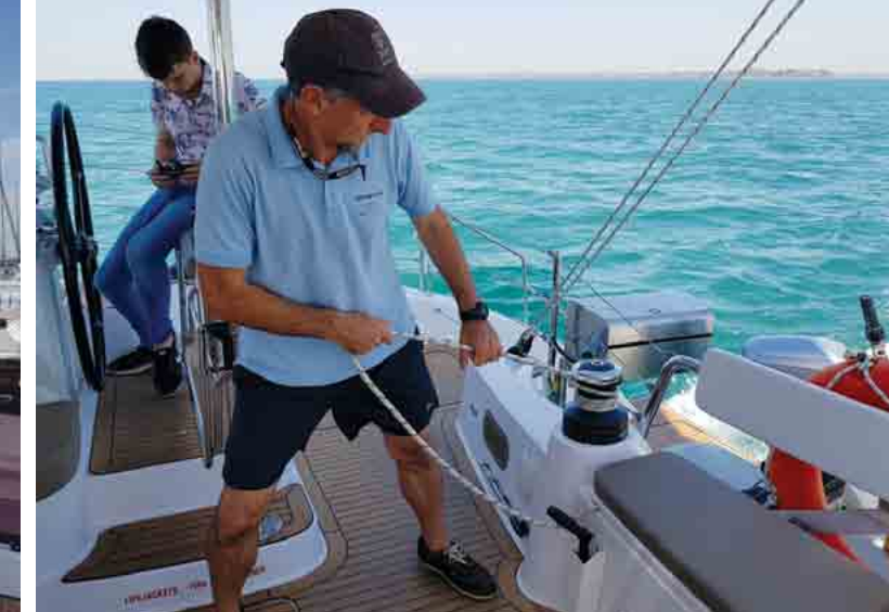
Twin outboard H50 winches easily controlled the mainsail and there was a preventer inbuilt to the boom as well. Image Kevin Green
