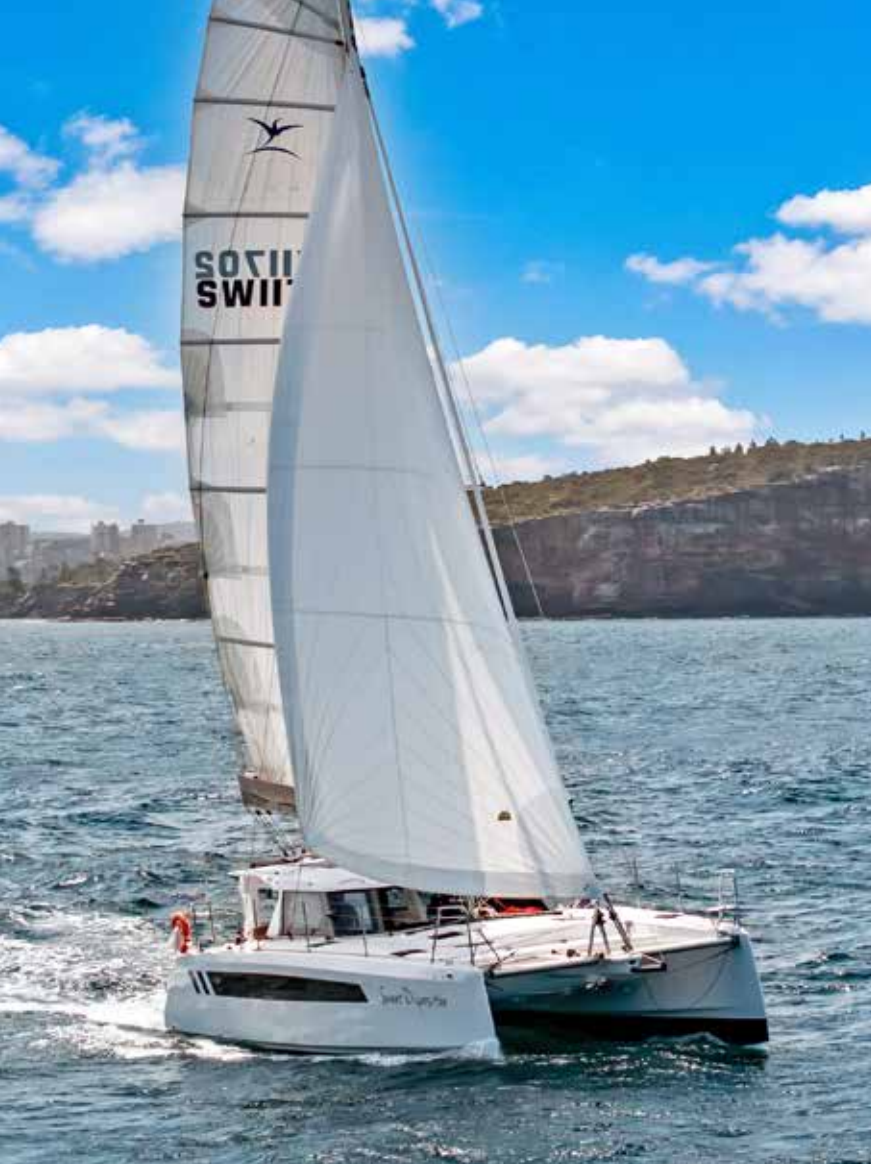
Above: Tall topsides, reverse bows and a raked-back coachroof reflect European styling.
